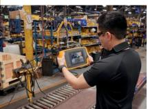
The ii900 Sonic Industrial Imager lets technicians see sound as they scan hoses, fittings and connections for leaks. Its built-in acoustic array of tiny sensitive microphones generates a spectrum of decibel levels per frequency. Based on this output, an algorithm calculates a sound image, known as a SoundMap, which is superimposed on a visual image. The SoundMap is automatically adapted, depending on the frequency level selected, so that background noise is filtered out.
