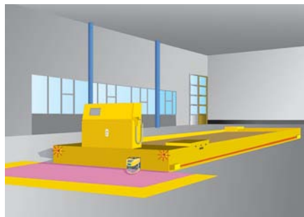
Lateral protection on an automated guided vehicle
